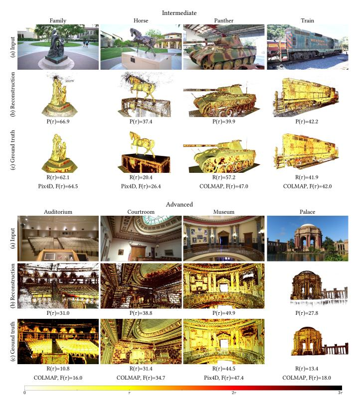
Fig. 5. State-of-the-art results on a number of benchmark datasets. (a) A frame from the input video sequence. (b) Reconstruction produced by the bestperforming pipeline, with distance to the ground-truth model coded by color. (c) The ground-truth model, with per-point distance to the reconstruction coded by color.
